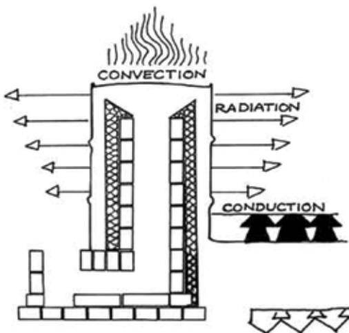
top uppermost. The chamber burns small-diameter wood in a remarkably efficient way; the barrel contains and channels the combusted gases whilst the surfaces radiate and conduct heat into the room. Wood gases, after burning forcefully in the burn tunnel and riser, are then 'pushed' down the inside of the barrel and channeled into a duct made from metal or brick. This duct can run to lengths of 30 feet before a chimney vents to outside. Sounds impossible? I assure you it's true!
